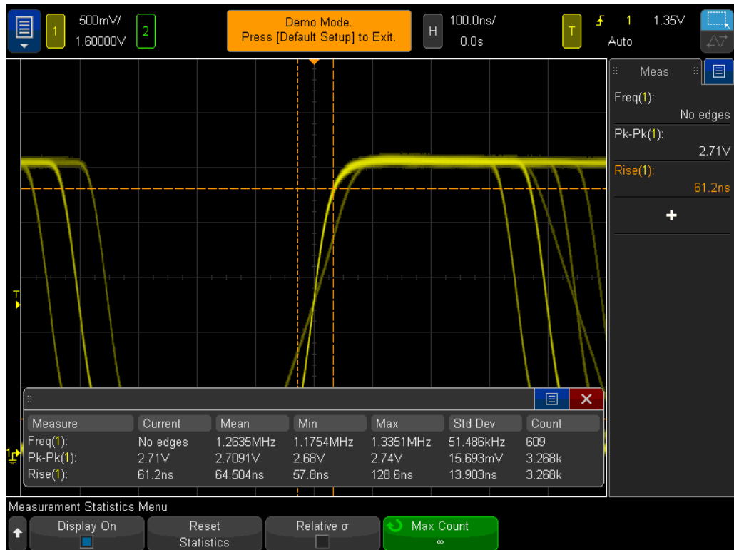
Figure 32 The scope's measurement statistics shows the range of rising edge speeds on this signal.
