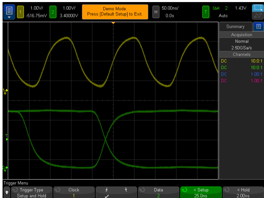
Figure 42 Triggering the scope on just setup time violations of less than 25 ns.
