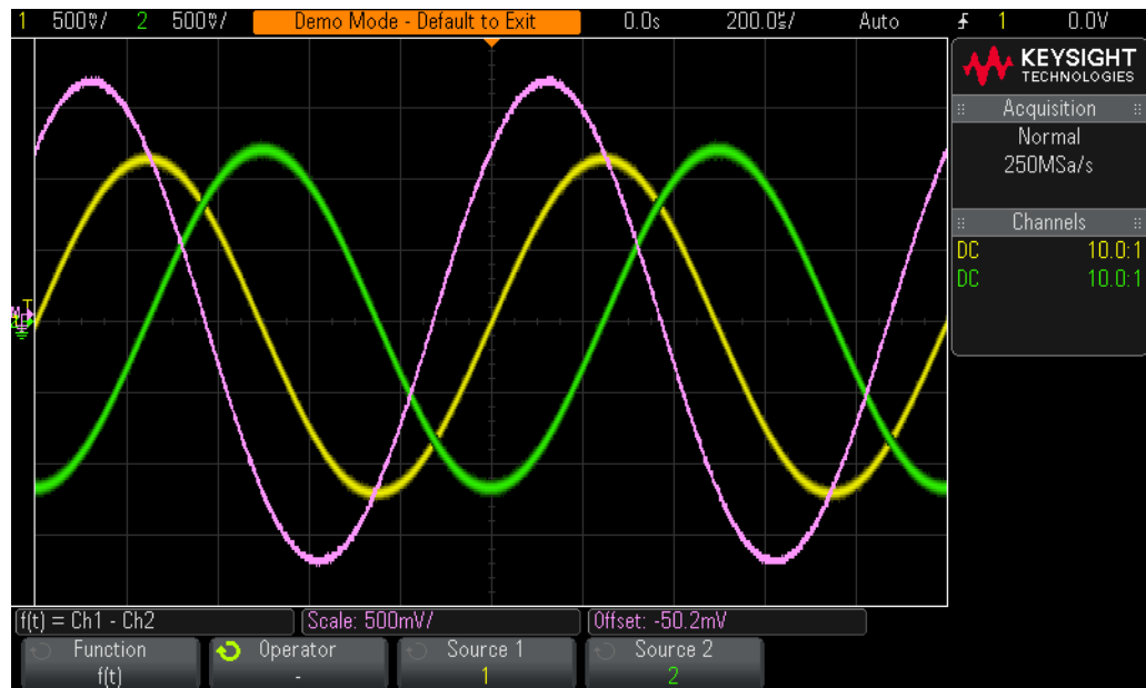
Figure 11 Using waveform math to subtract channel-2 from channel-1.
