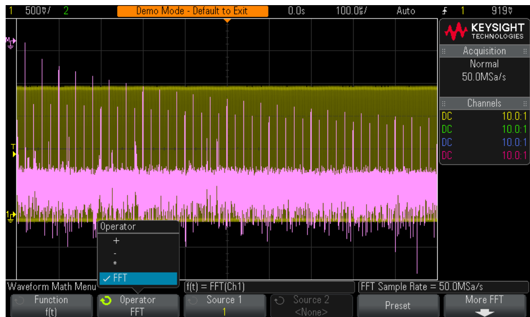
Figure 43 Performing an FFT math function on a repetitive digital clock
