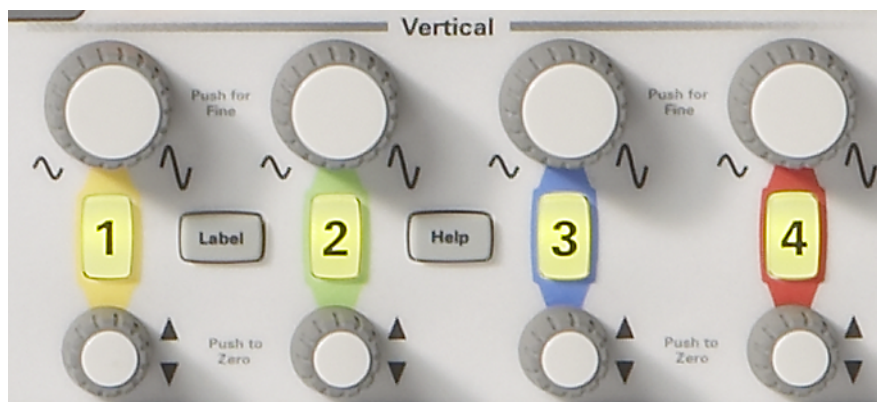
Figure 5 Oscilloscope vertical (Y-axis) controls
