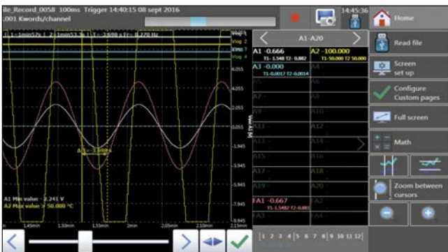
Measurement display with zoom and cursors
