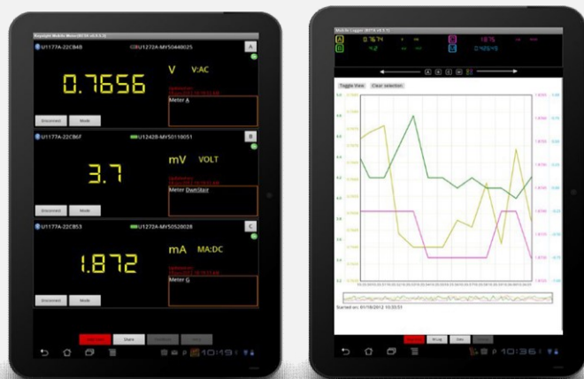
Figure 3. Once connected to any HH DMM via Bluetooth adapter you are able to log and view measurements graphically from smart phones and tablets.
