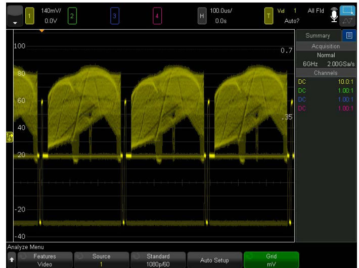
Figure 45. Triggering on a 1080p/60 signal.
