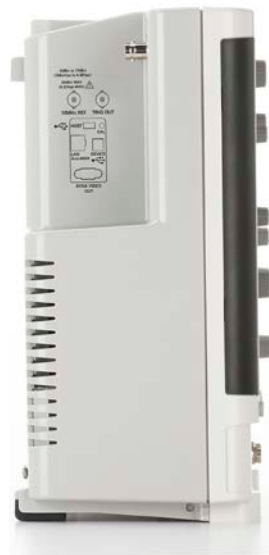
Figure 8. One-gigahertz-per-inch form factor: 6 GHz, 6 inches deep.
