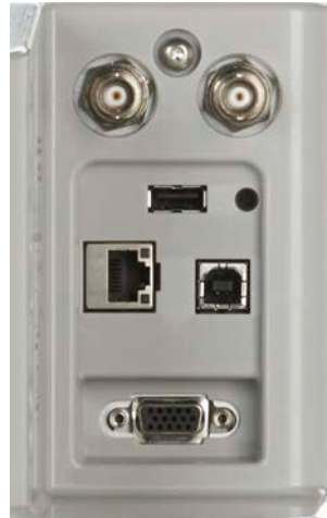
Figure 52. Connectivity section on the back panel.
