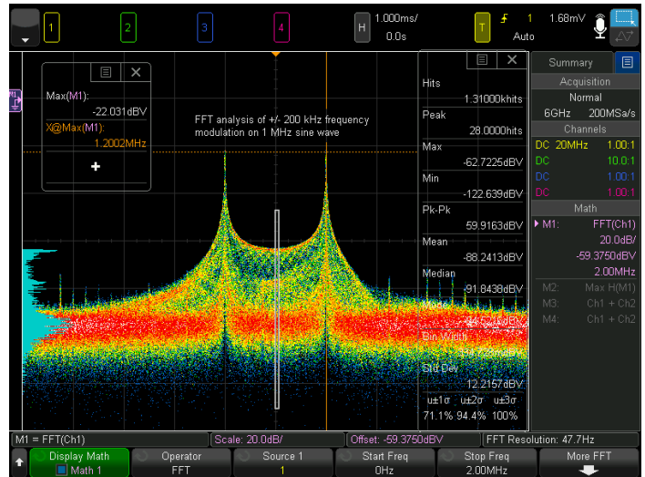
Figure 16a. Color grade and histogram on an FFT function.
