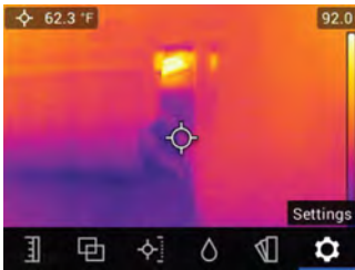
Figure 5.1 Main Menu icons at bottom of display. Press Select to reveal the icons.
