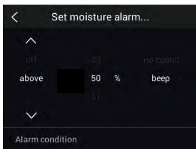
Figure 7.13 Setting the Moisture Alarm
