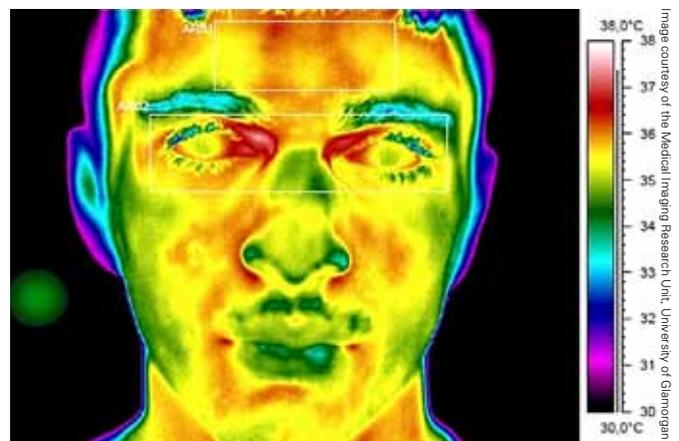
FLIR IR cameras automatically detect elevated skin temperatures that may indicate a fever and underlying infection. Each camera's unique Automatic Temperature Compensator (ATC) adjusts for ambient conditions to minimize false readings. The color image, temperature scale, and alarm mechanism make it easy to decide when a person needs further examination.
