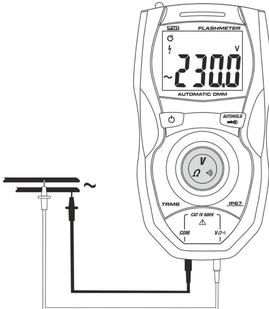
Fig. 4: Use of the instrument for AC voltage measurement
