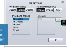
RTD can be connected with 2,4 or 4 wires and you can select various tables such as the IEC 60751, JIS or Callender Van Dussen
