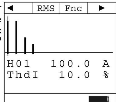
3. Press **F3 (Fnc)** to open the drop-down menu shown on the screen aside. At each subsequent pressure of key **F3**, the cursor will scroll through the available items as follows:
