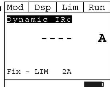
3. Press **F2 (◀)** or **F3 (▶)** to set the reference threshold for the saving of event (**2A ÷ 100A** for “Inrush 100A” and **5A ÷ 900A** for “Inrush 1000A”)
