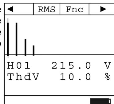
3. While measuring Voltage Harmonics, press **F3 (Fnc)** to open the drop-down menu shown on the screen aside. At each subsequent pressure of **F3**, the cursor will scroll through the available items, as follows:
