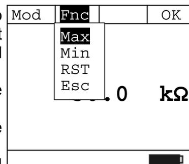
12. Pressing **F4 (OK)**, the selected item is confirmed. Nearby, an example of measurement with active Max function. The display shows the active function.
