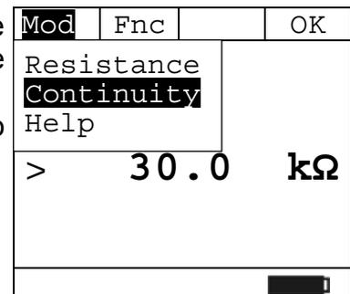
8. Press **F3(Lim)** key to set the limit value of Continuity test (if the measured resistance is lower than the set limit resistance value (e.g. Res Lim: 1Ω), the buzzer sounds continuously).
