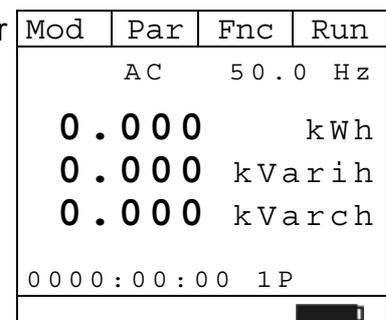
18. Press **F4 (Stp)** to stop the energy measurement. The corresponding value is displayed. Press **F4 (Run)** again to zero the counter and start a new energy measurement.
