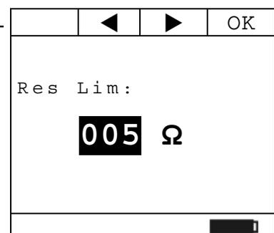
11. While measuring Resistance or Continuity, press **F2 (Fnc)** to open the drop-down menu shown on the screen aside. At each subsequent pressure of **F2**, the cursor will scroll through the available items, as follows:
