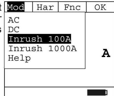
2. Press **F3 (Lim)** for the setting of limit threshold value on inrush current and the type of measurement as shown asides
