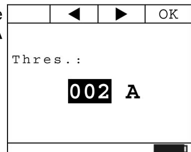
5. Press **F4 (Run)** key to start the detection of the inrush current event. Press **F4 (Stp)** to stop the detection of the inrush current event in any time. After the detection of the event (when the measured current is over the limit threshold), **the measurement is automatically stopped** by the instrument and the maximum RMS value in 100ms is displayed as shown asides
