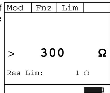
9. Press **F2 (◀)** or **F3 (▶)** and set the limit value within the **1Ω ÷ 150Ω** interval
