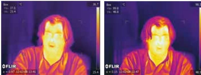
The thermal image on the left has the right emissivity settings for human skin (0.97) and the temperature reading shows the correct temperature (36.7 °C). For the thermal image on the right, the wrong emissivity was entered (0.15), leading to a false temperature reading (98.3 °C).
