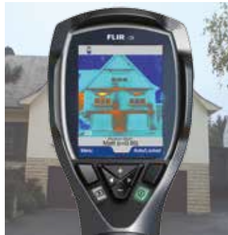
FLIR i3, temperature in 3,600 spots
