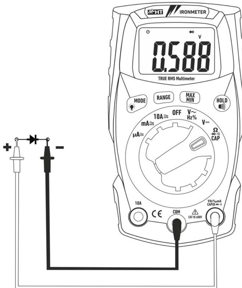
Fig. 6: Use of the instrument for diode test
