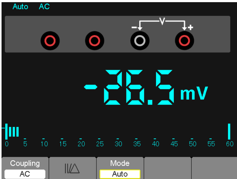
Figure 7-7 AC voltage Measurement
