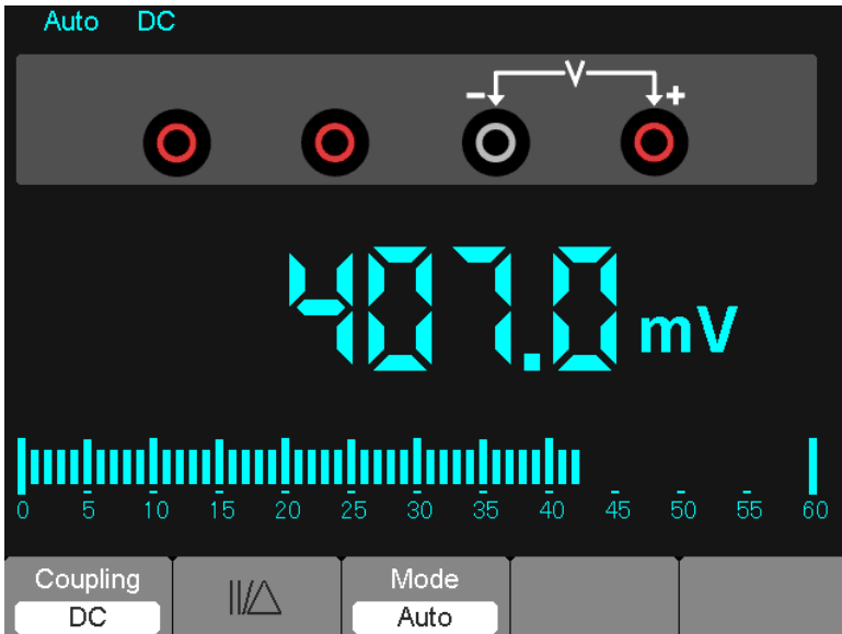
Figure 7-6 DC voltage Measurement
