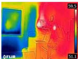
Uninsulated outside wall
